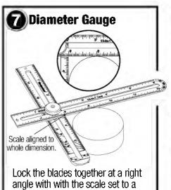
whole dimension. Now, read the thin gauge where the blade touches the round object and calculate your radius. Double it for your diameter.
