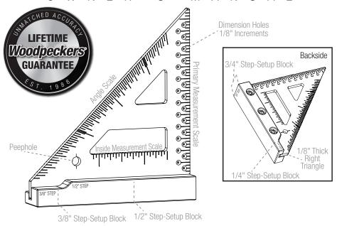
The ingenious **Woodpeckers DelVe Square** was originally developed by North Carolina professional woodworker, Tom DelVecchio. Tom and our product developers have updated the design with a stainless steel blade, 1° increments on the angle scale and precision milled setup block sections. Take a few minutes to review this Owner's Manual to familiarize yourself with the unique features of your new DelVe Square.
