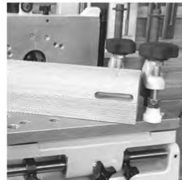
FIGURES 14. Use the "X" and "Y"-axis control arms to bring the horizontal table forward and left-to-right to cut your mortise.
