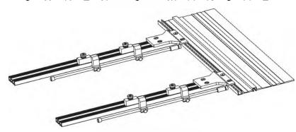
**Woodpeckers Parallel Guide System (PGS)** provides effortless repetitive cuts when paired with Festool's\* Guide Rail and Track Saw. Using a physical stop, just like a table saw rip fence, each cut is exactly the same as the one before.
