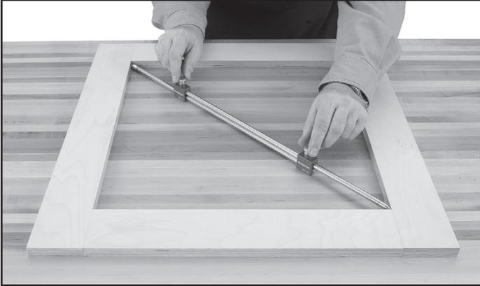
Attach **Arrow Tips** to check if a cabinet, frame or drawer box is square by comparing the distance between diagonal corners.
